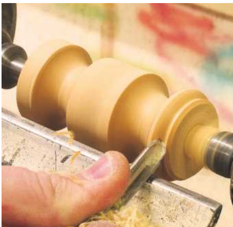
▲ Pic.25 Les is going to do this end with the gouge, keeping the bevel in the direction of cut. You can work down until there is as little as 3mm of timber supporting the end
